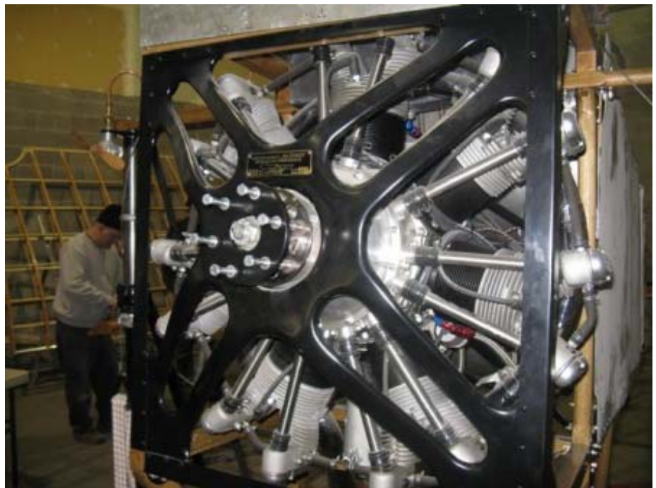
The black former in front of the engine is hand formed from aluminum. Note dataplate above prop hub – see zoomed view below
